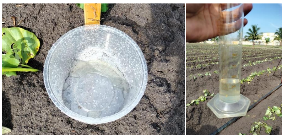
Figure 3. Volumetric method (catch can and measuring cylinder)
