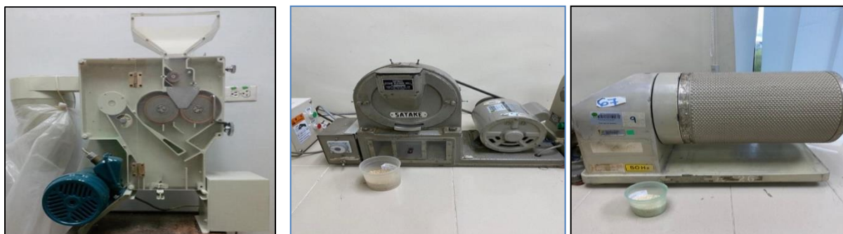
Figure 1: Laboratory scale instruments (dehussing, polishing and cylinder grading machines) used to obtain MRR and HRR
