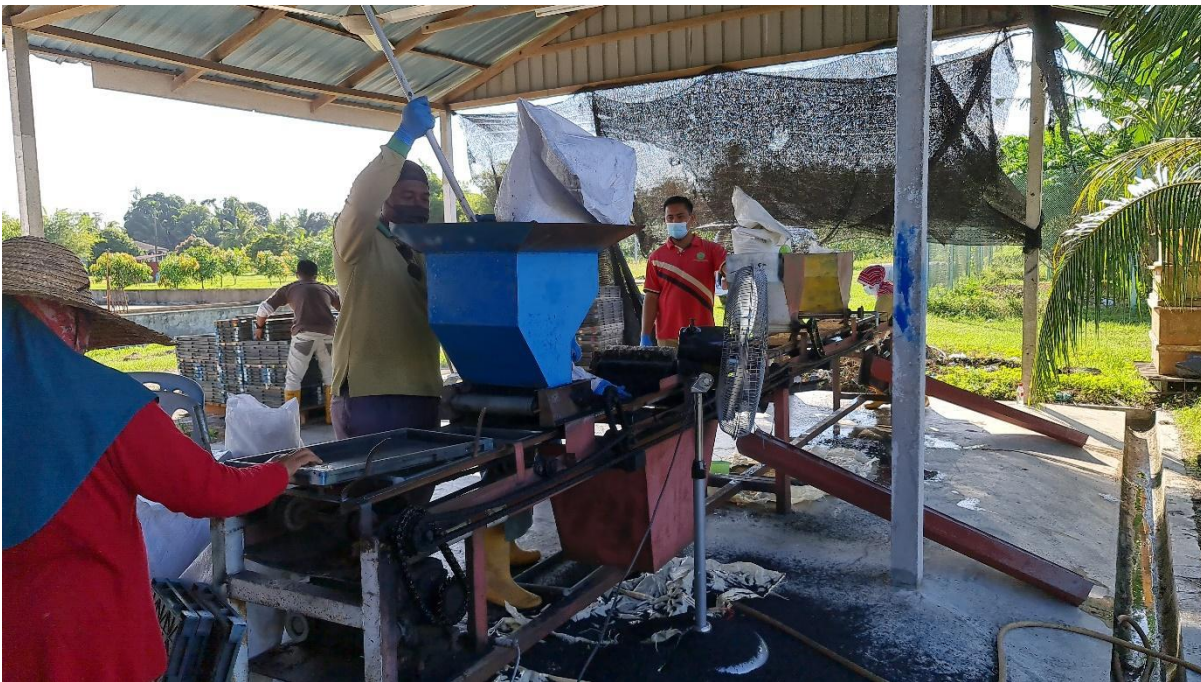
Figure 1. Rice tray seeding machine used.
