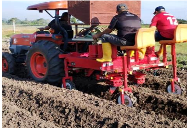
Figure 4. Tractor Kubota L4400 attach to two-rows pineapple transplanter
