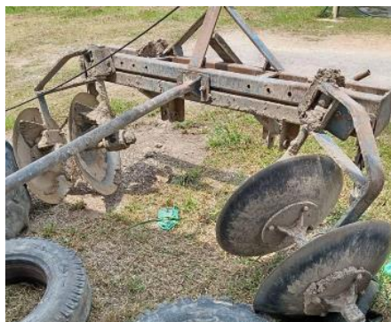
Figure 1. Raised bed with 4-disc conventional disc ridger implement.
