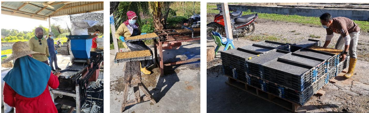
Figure 5: workers performing task at tray feeding, tray stacking and delivery to pallet.
