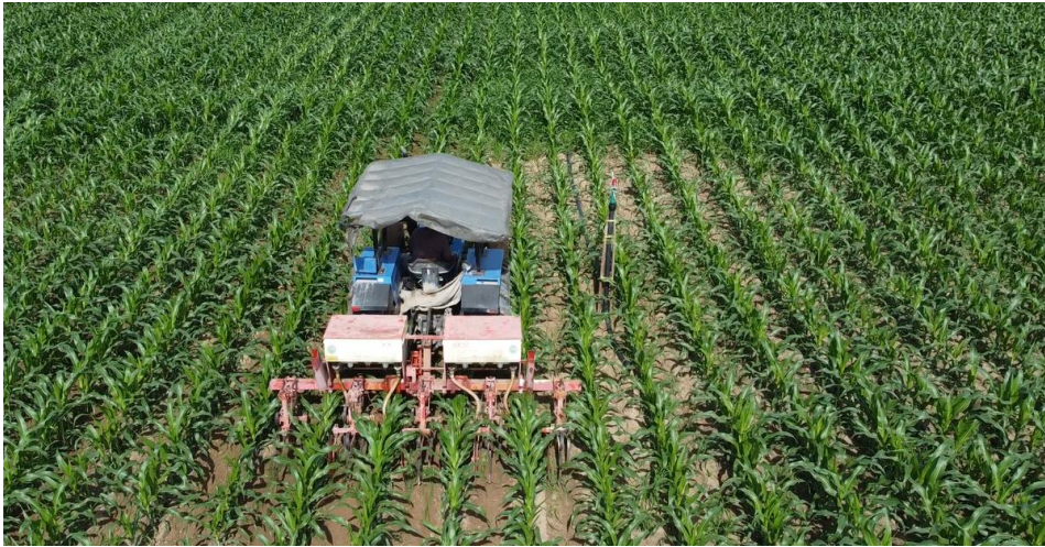
Picture 4. Secondary fertilizer application with a spreader machine between the boundaries with fertilizer application system mounted on a tractor.
