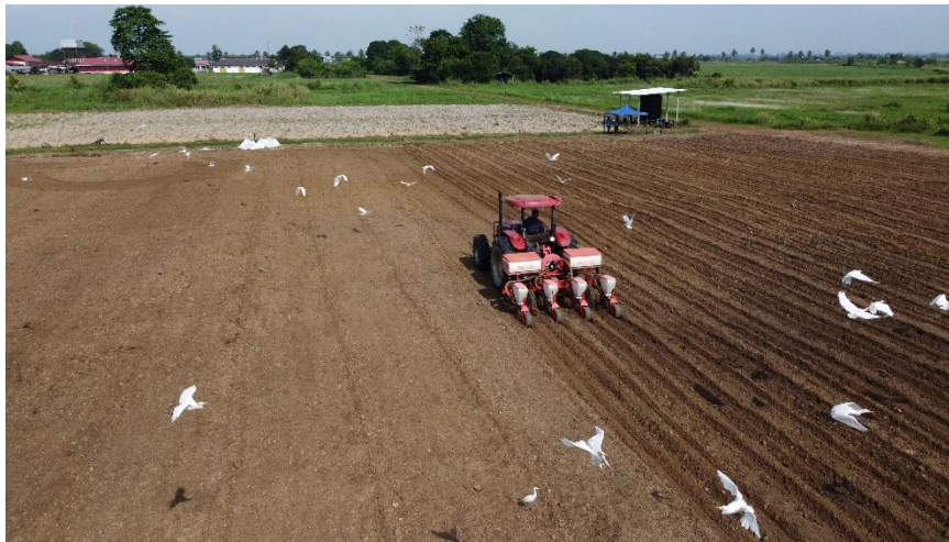
Picture 1. Pneumatic system seed nursery machine (Gaspardo type) tractor attachment equipped with four rows of seed seeder with feeder fertilizer.
