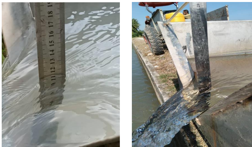
Figure 6. The ruler soldered v-notch
