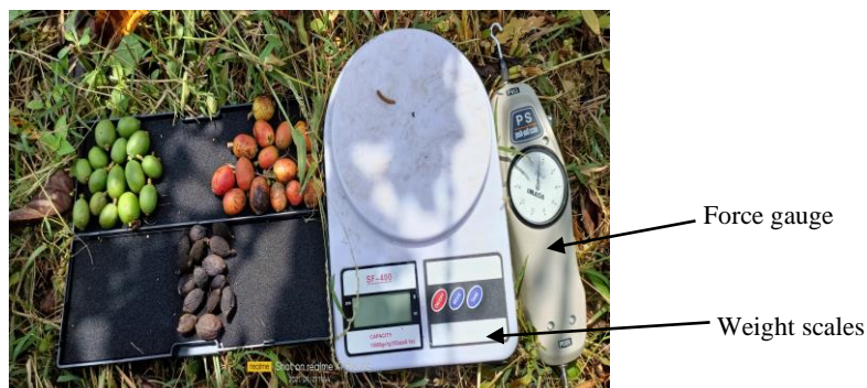
Figure 2. Measuring force load and strength using force gauge and weight scales
