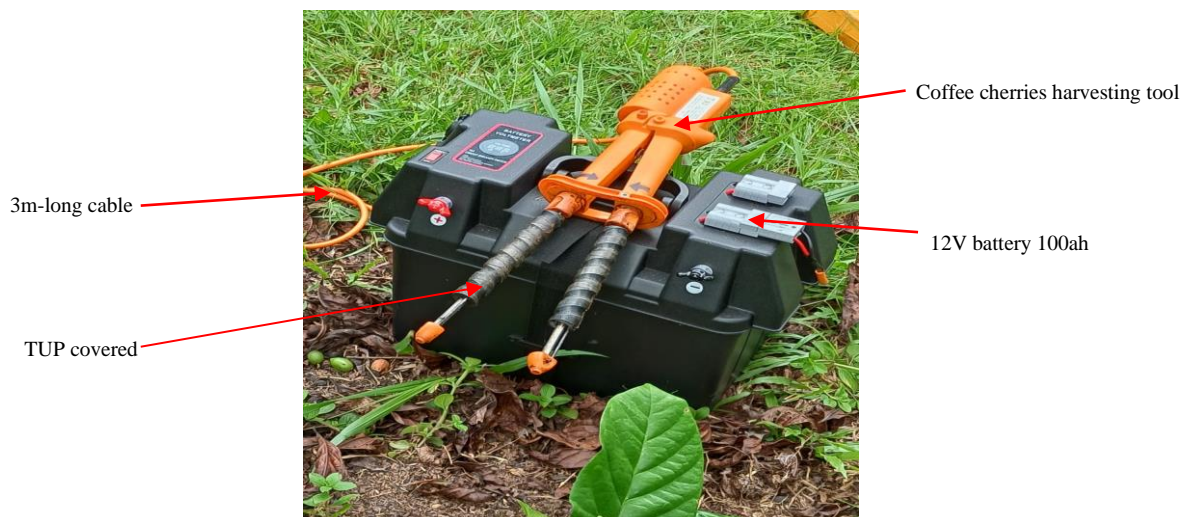
Figure 3. Coffee cherry harvesting tool with 12V battery 100ah
