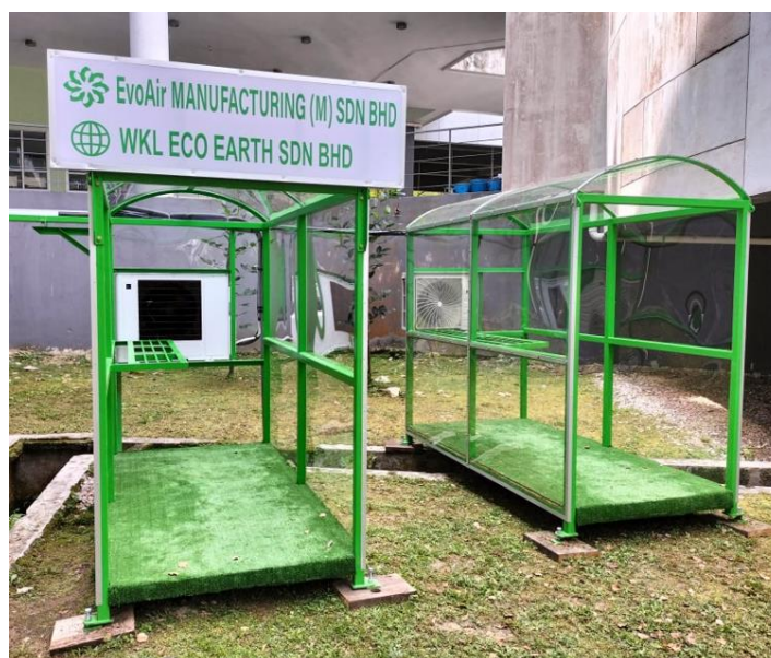
Figure 1: Two green houses were constructed to receive hot air/heat generated from the two different brand’s condensing unit (i) Evoair, (ii) Control
