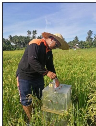
Figure 2: Gas sampling process at the field
